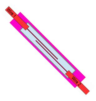
It's tricky to insert the wires correctly. You want to make sure that both metal wire tips are inserted fully into the inner metal sleeve inside the Barrel Connector. The exposed metal of Wire 1 and Wire 2 should be fully inside the inner metal sleeve: Yeah it's hard to describe but look at the diagram above.
