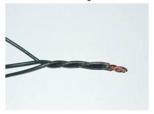
Use a Wire Nut to twist onto the metal tips. Try the small or medium size wire nut in your variety pack. Quick video lesson:
