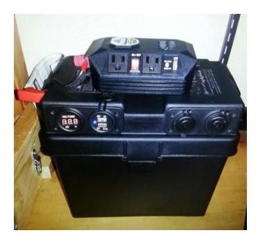
At the very least, make sure the inverter is in the shade and not sitting in a pile of dust.
