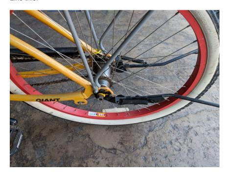
You will need some muscle to pry apart the sides of the kickstand a bit, and fit the kickstand slots over the bolts on each side of the rear wheel.
