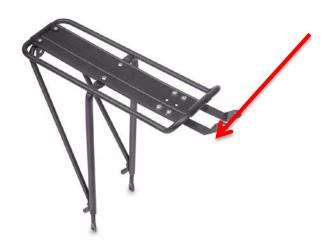
Then attach the lower legs of the rack to the rear hub/frame. It's normal to have to pull the rack legs open a bit to get it to fit. Typically the rack legs go on the OUTSIDE of the bike frame. But do whatever works for your bike.
