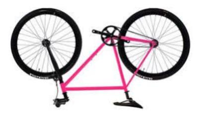
Take off the rear wheel nuts (you'll need wrenches), but you can leave the wheel on the bike. If you have a quick-release rear wheel, just open the quick-release and then unscrew both nuts a few times on each side of the wheel to loosen them.
