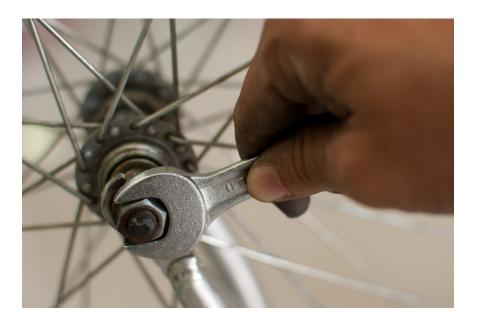
If it's a cruiser bike, you may need to loosen and/or remove the nut on the coaster brake too:
